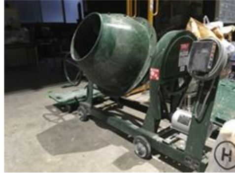
Fig.3 Tilting mixer used during mixing and low speed agitating
