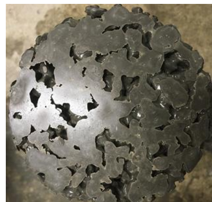
Fig.5 Condition of paste on the bottom of the specimen (HAE/C=0.4%, 0 minutes after mixing)
