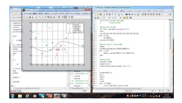
sounds. SVM need multiple features to distinguish sounds. Choose features decide efficiency of system. As it is very difficult, I couldn't choice appropriate features. First feature is found using wavelet transformation to know behaver of frequency. Second feature is sound pressure. I thought that there are relation of frequency and sound pressure.
