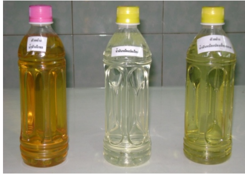
Fig. 5 Diesel oil, transformer oil and transformer used oil
