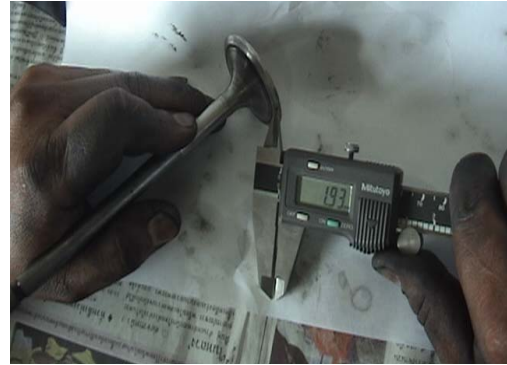
Fig. 7 Inlet valve measurement
