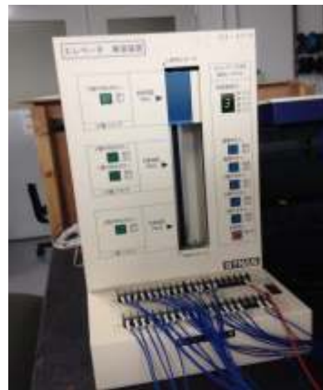
I have been practiced simulated the elevator signal control
